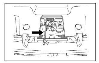
2. Then go to the front of the vehicle and locate the secondary hood release, near the center of the grille.
